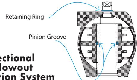
The anti-blowout system of the pinion is ensured thru a double protection: both with an upper c-clip and two keyways casted on the pistons. In case of unusual downward movement of the pinion, the keyways will interfere with the grooves on the pinion and therefore stopping it.
