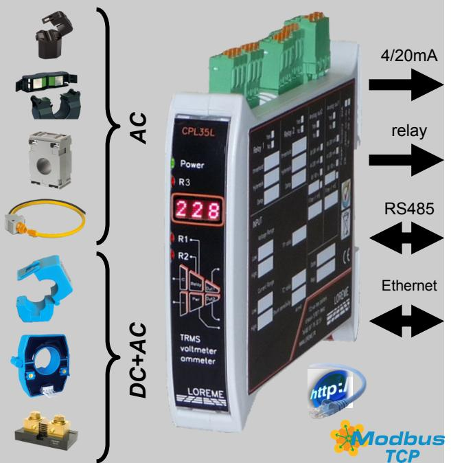
The CPL35L is a programmable voltage and current transducer. The various output options allow a wide range of application: measurement, protection, control. The second analog output allows simultaneous measurement of voltage and current in total isolation.
