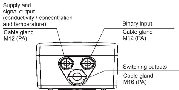
**Wiring recommendation - with separate sensor**
