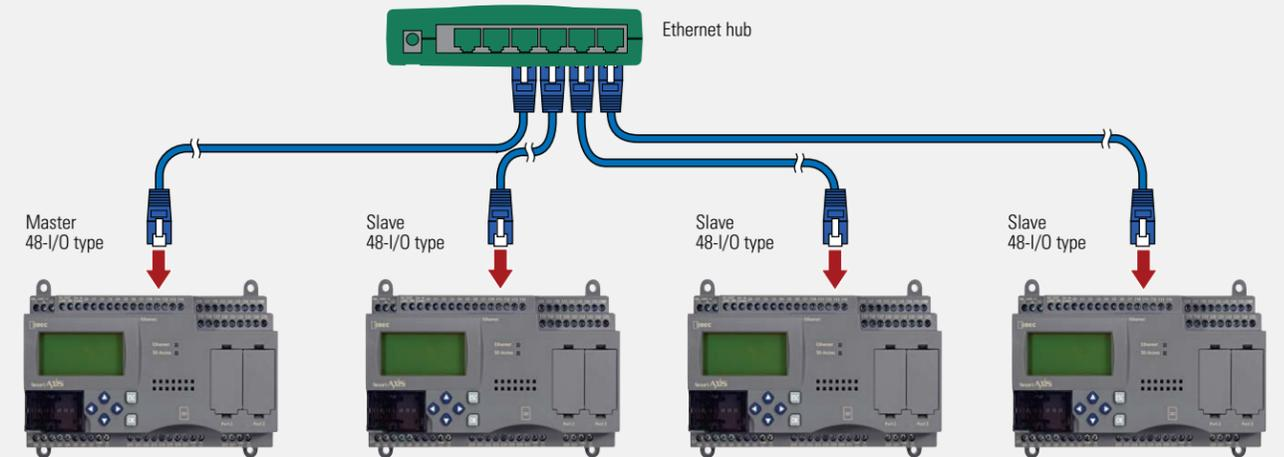
48-I/O type (master) + 48-I/O type (slave) + 48-I/O type (slave) + 48-I/O type (slave) = 192 I/O
