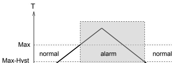
A switchover delay time ( $t_{DS}$ ) can be applied to the switchover to the alarm state. Equally, one switch-back delay time ( $t_{DR}$ ) of several can be applied to switching back to the normal state.
