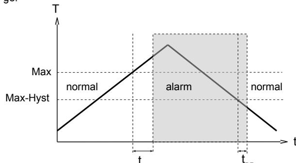
In the non-inverted (standard) model, while in the normal state the switching output is at the level of the supply voltage; in the alarm state it is at 0 V, so that a wire break would also display as an alarm state at the signal receiver. Optionally, an inverted switching output can also be provided, i.e. in the normal state the output is at 0 V, and in the alarm state it is at the level of the supply voltage.
