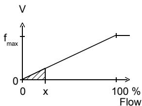
$f_{max}$  selectable in the range of up to 2000 Hz
