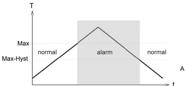
switchover delay time ( $t_{DS}$ ) can be applied to the switchover to the alarm state. Equally, one switch-back delay time ( $t_{DR}$ ) of several can be applied to switching back to the normal state.
