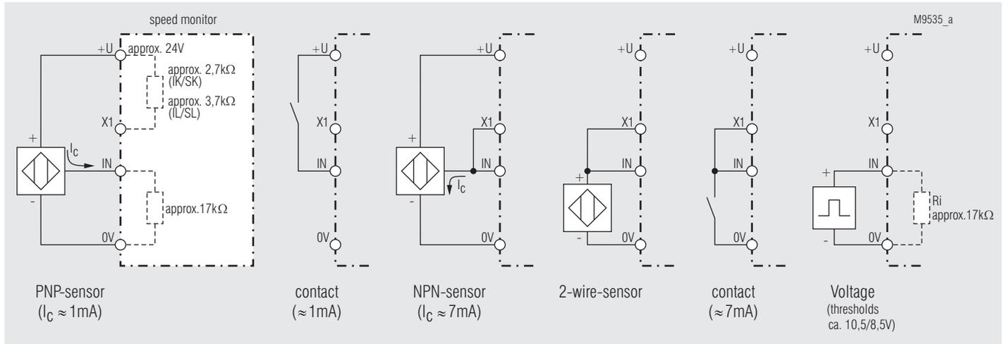
Note: For IK-models the auxiliary voltage (DC 24 V) must be additionally connected to terminals +U/0V
