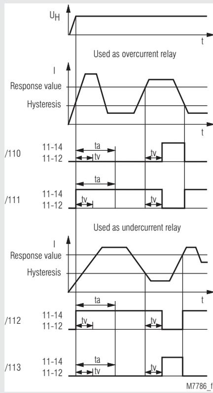
On model BA 9053/6\_ with manual reset the contacts remain in the fault state after detecting a fault or after  $t_o$  has elapsed. The contacts are reset by disconnecting the supply voltage.
