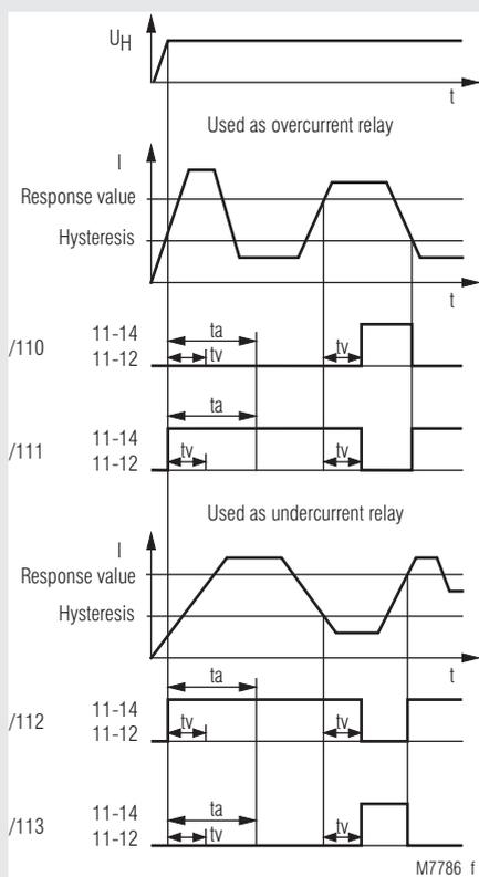
On model MK 9053N/6\_ \_ with manual reset the contacts remain in the fault state after detecting a fault or after  $t_a$  has elapsed. The contacts are reset by disconnecting the supply voltage.
