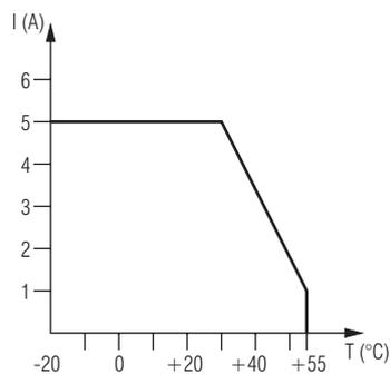
Continuous current limit curve (Current over 2 contacts)
