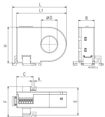
For DIN rail mounting or screw mounting
