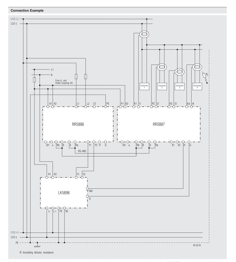
Insulation monitoring and insulation fault detection with 4 connected measuring current transformers in a AC (DC) - network with subdistribution - insulation fault detection can be controlled by the insulation monitor /LK 5896); bus termination of the first and last device on the RS-485 bus.
