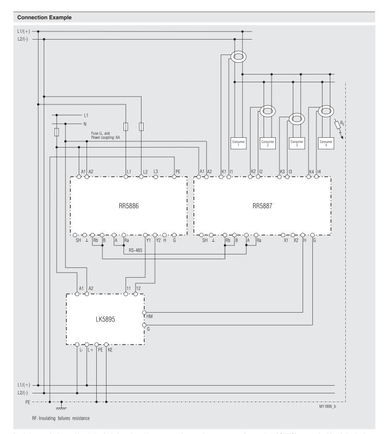
Insulation monitoring and insulation fault detection with 4 connected measuring current transformers in a AC (DC) - network with subdistribution - insulation fault detection can be controlled by the insulation monitor /LK 5895); bus termination of the first and last device on the RS-485 bus.
