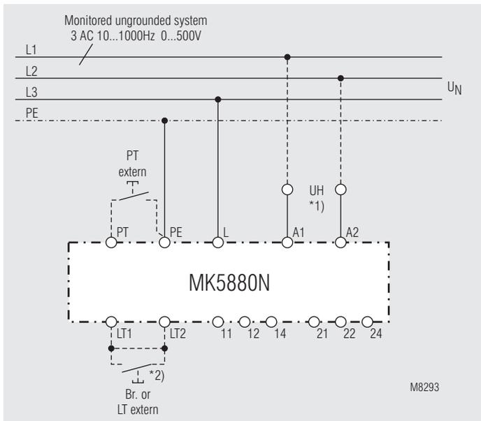
Monitoring of an ungrounded voltage system.
