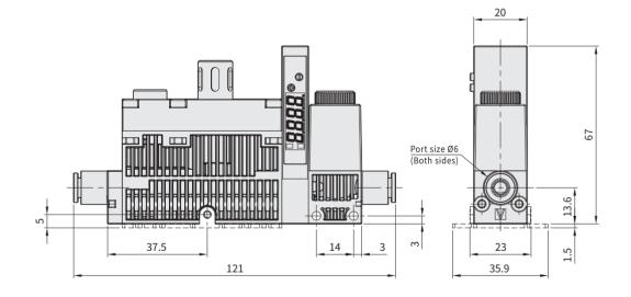
• Note: The product is without vacuum breaking, the breaking air source should be set up separately.
